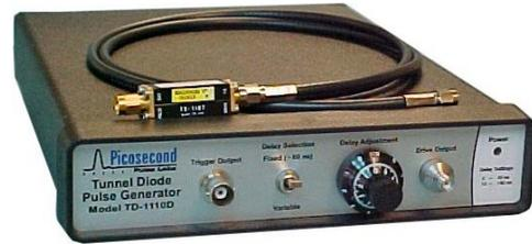
The Tunnel Diode Pulse Generator consists of the Model TD1110D Driver with a TD1107C Pulse Head. This combination produces a 230 mV step with risetime in the range of 20 ps to 25 ps. The 50-ohm source impedance minimizes reflections. The Tunnel Diode Pulse Generator may be operated into any unbiased, resistive load without damage. Applications include Time Domain Reflectometry (TDR) and step response measurements on components.
